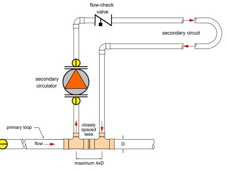
The secondary circuit is "hydraulically separated" from the primary circuit by the closely spaced tees.
