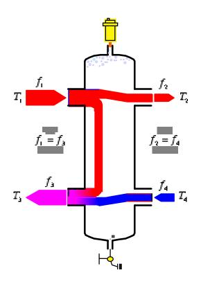
Heat is being injected faster than the load is removing heat.
