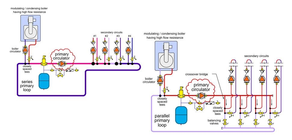
This adds to the installed cost of the system **AND** add hundreds, even thousands of dollars in operating cost over a typical system life.
