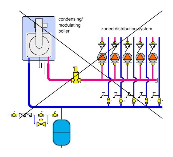
The solution to this problem is **hydraulic separation**. In short, preventing flow in one circuit from interfering with flow in another circuit.
