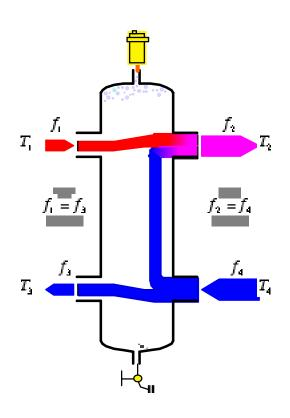
The mixed temperature (T<sub>2</sub>) supplied to the distribution system can be calculated with:
