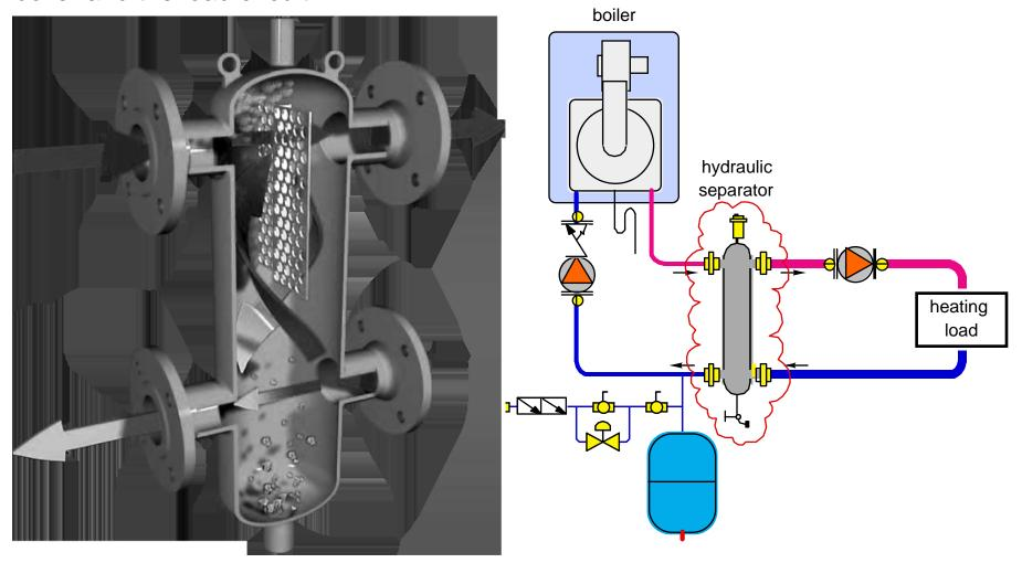
The low vertical velocity inside the separator produces minimal pressure drop top to bottom and side to side. This results in hydraulic separation between the boiler circuits and load circuits.
