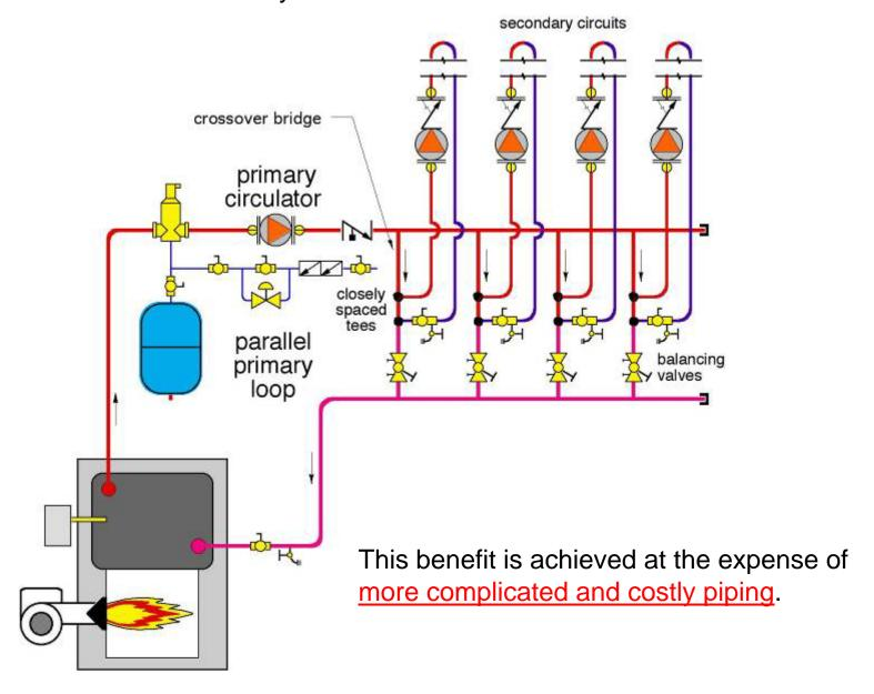
In addition, both **series** and **parallel** primary/secondary systems require a <u>primary circulator</u>.
