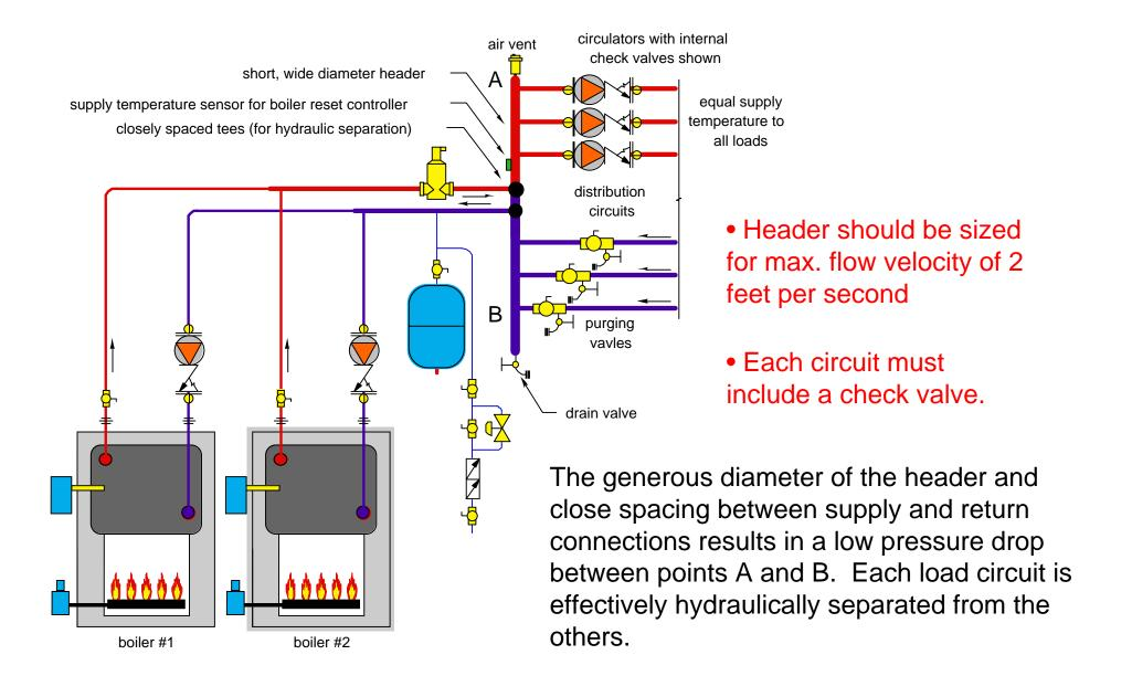
Another option is a specialized component called a *hydraulic separator* between the boiler and the load circuit:
